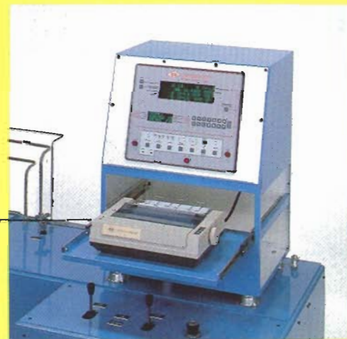
Figure 3 Bead Unseating Fixture in Place for Conducting Unseating Test
