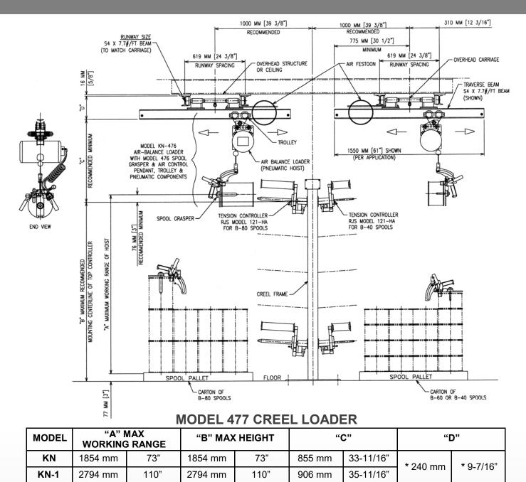
\* USING S4 x 7.7 #/FT BEAM FOR RUNWAYS AND TRAVERSE BEAM
