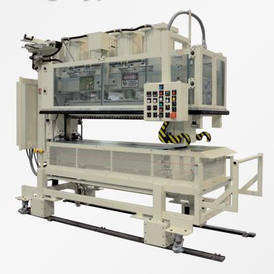
to close until the guard is completely closed. Two hooks prevent deflection of frame when pressing. The movement of the hooks and press are interlocked.
