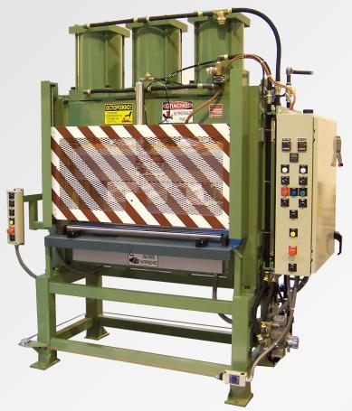
The Model 344 Splice Press is employed in the steel cord calendering process, and is used for splicing the trailing ends of steel cords from a completed creel run to the leading ends of cords from a newly started creel run.
